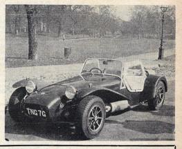
LOTUS SEVEN TWIN CAM 'S' Specification includes Lotus Holbay 125-b.h.p. twin-cam engine, Elan +2 'S' gearbox, 3.9 limited slip differential, Lotus alloy wheels, redesigned fascia, instruments, and trim, at £1,225 in component form.
