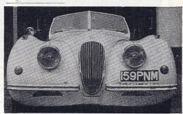
1950 JAGUAR XK120 roadster, rebuilt with the following specification. 3.4-litre engine, with the 4.2-litre gearbox and constant mesh starter. White coachwork, rechromed throughout and fully retrimmed in red Connolly hide with red carpets. Koni shock—absorbers, 15in. 'E' type chrome wire wheels and whitewalled radial tyres. £1,745.
