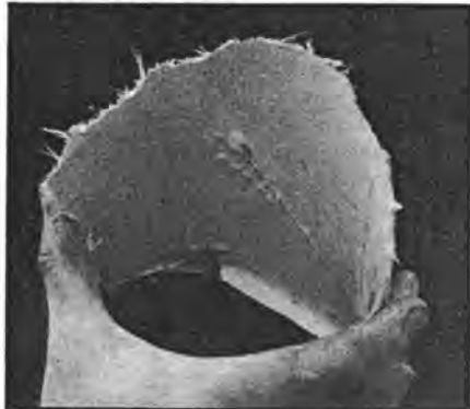
Overflexing will cause cracks and paint splitting.
