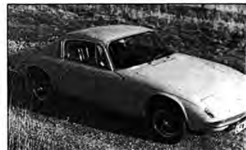
The final result. All the body was stripped and repaired and 16 coats of colour applied, flatted off after every four and finally hand-polished.
