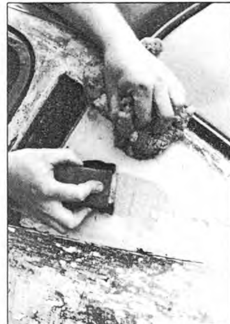
Flattening off by hand with 220 grade paper back to bare GRP on this three-quarter panel. Sponge is squeezed to supply a constant dribble of water. Eventually the whole car has to look like this.
