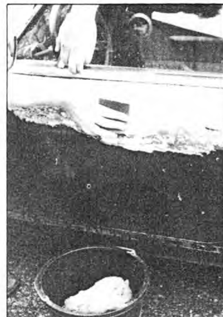
Flattening the area by hand down to the bare GRP.
