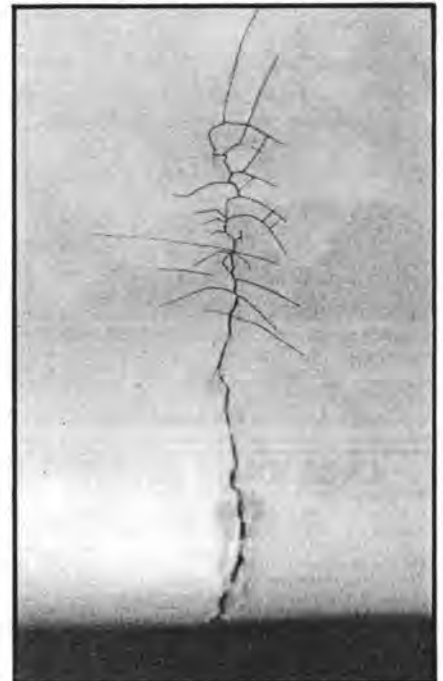
Extent of crack travel from a nudge on a wheel arch.
