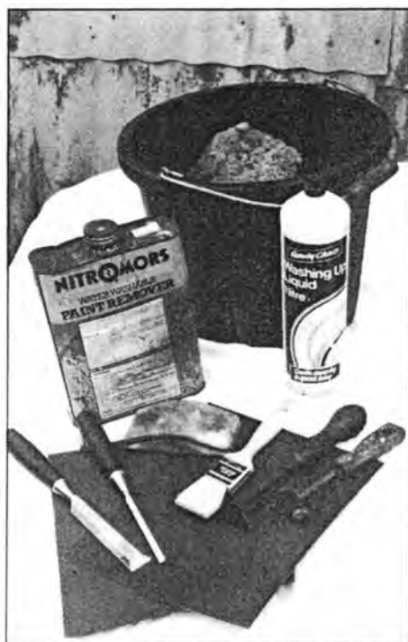
Essential equipment: Paint remover, chisels, multi-sided scrapers, wet and dry papers, bucket, sponge and washing up liquid.
