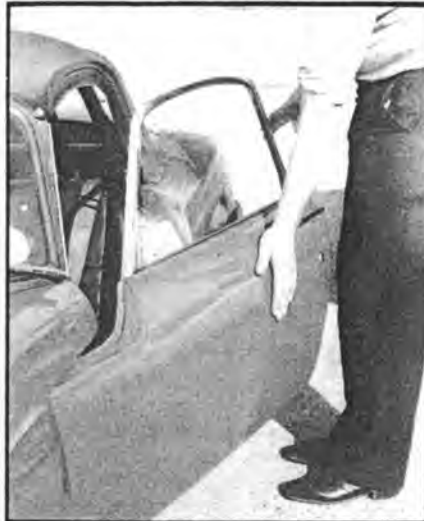
How to shut a door properly with a hand flat against the panel to spread the minimum force necessary over as large an area as possible.
