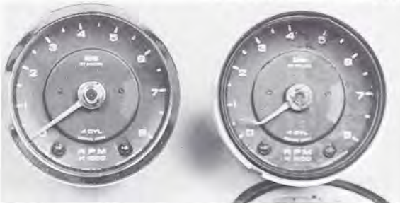
This shows after/before typical instrument overhaul service.
